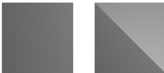
Figure 3.25: Figure depicts the planar and non-planar tetragon rendered by Blender engine. Notice, that the non-planar tetragon was automatically divided by Blender into two triangles.
